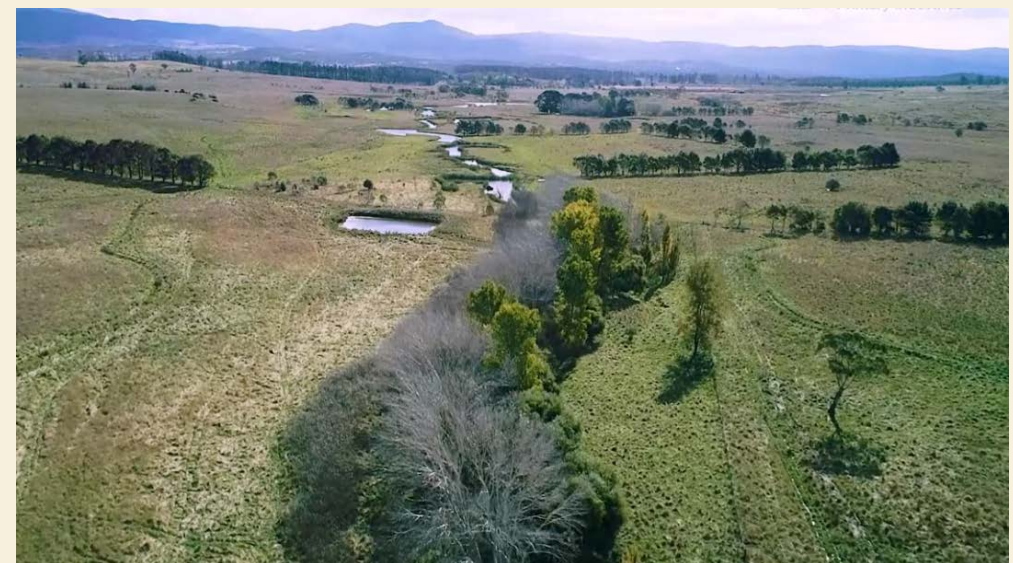
An aerial view of Martin Royds' 'chain of ponds', designed to slow water flow and rehydrate the soil.
